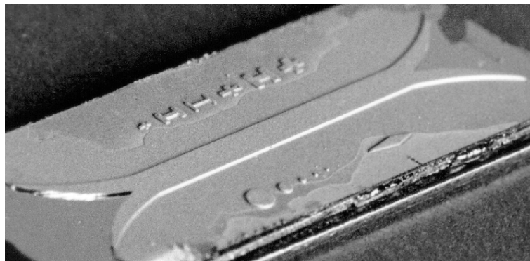
Figure 2. Photograph of Micro-machined Waveguide and Antennae.
